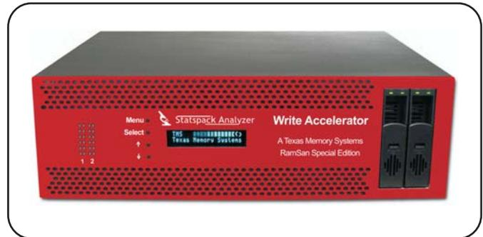
The Write Accelerator consists of two separate but bundled units, enabling complete support for SAME and allowing even the most demanding enterprises in the world 5-nines reliability for the solution. These two systems can be mirrored from the operating system or through Oracle's ASM.
